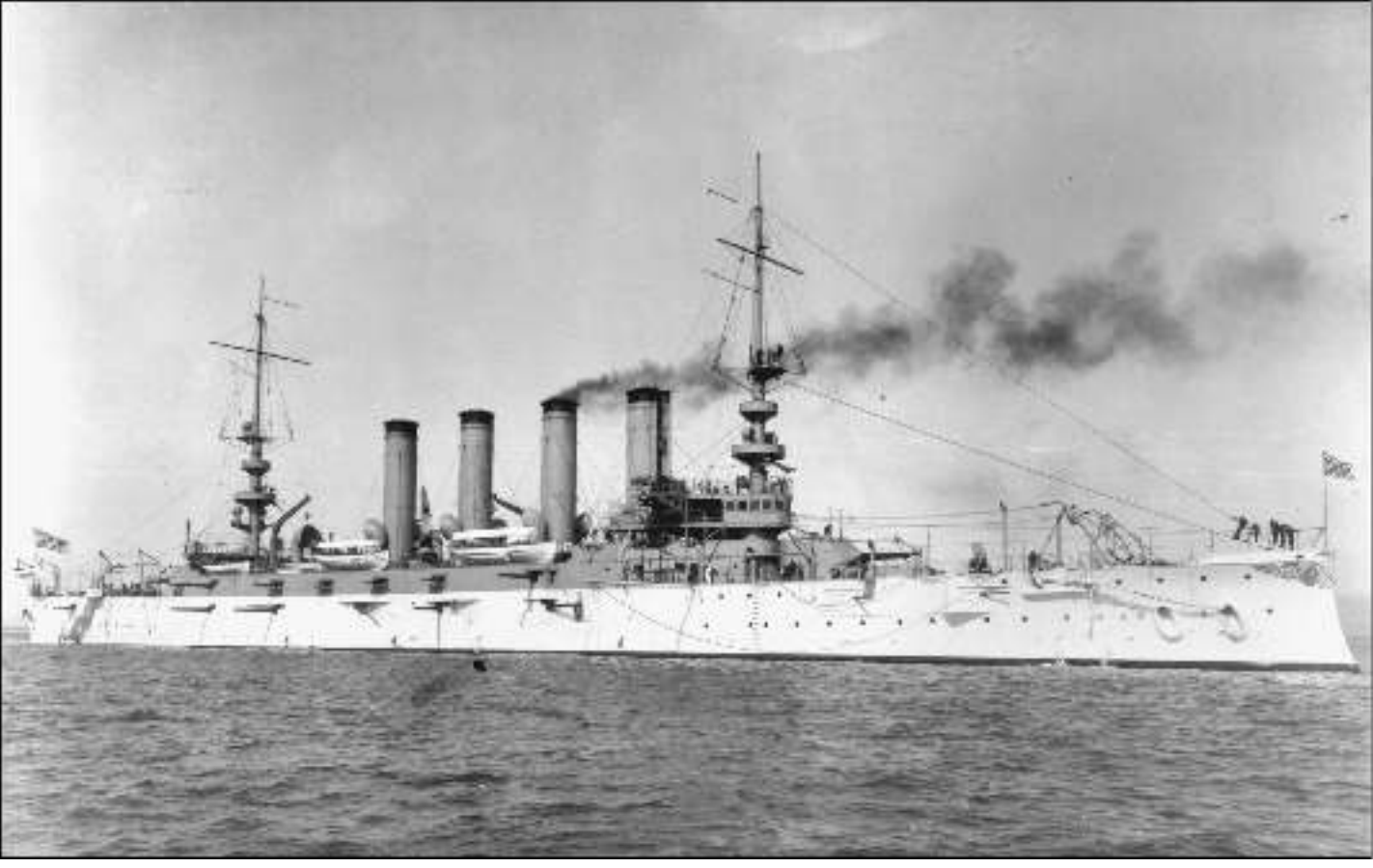
The armored cruiser San Diego was originally commissioned as California in 1907. This cruiser displaced 13,680 tons and was armed with four 8-inch and fourteen 6-inch guns, making her one of the most powerful ships of her kind in the pre-dreadnought era. California was renamed San Diego on September 1, 1914, so that the name California could be used for a new battleship. The San Diego frequently served as flagship for the commander in chief of the Pacific Fleet. While on duty with the Atlantic Fleet escorting convoys during World War I, San Diego struck a mine laid by the German submarine U-156 off Fire Island, New York. San Diego sank in 28 minutes, but with the deaths of only six men, she was the only major warship lost by the United States during the war. An impressive Bureau of Ships model of San Diego and artifacts collected from the wreck can be viewed today at the
