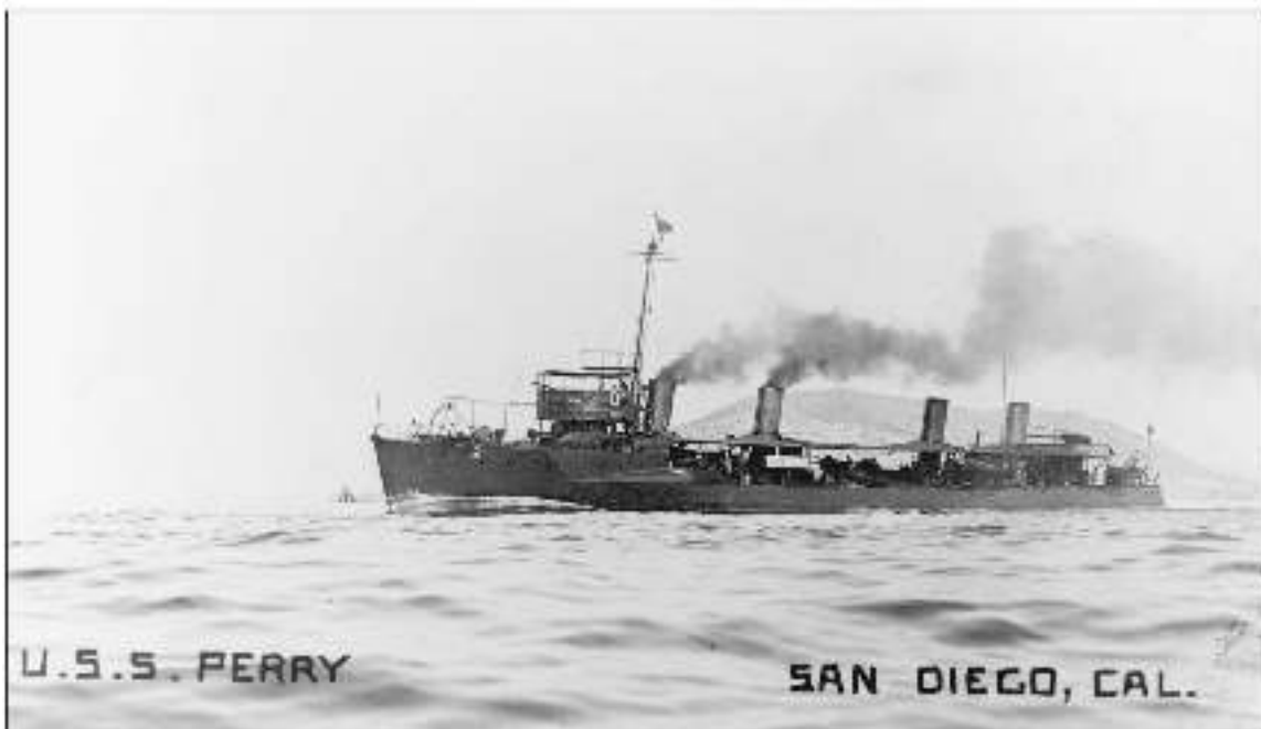
The sleek destroyer Perry, seen here leaving San Diego harbor c. 1915, is a good example of the first generation of destroyers built by the navy to combat the fast light-torpedo boat. Her open bridge, low freeboard, cramped quarters, and decks that were almost always wet all contributed to the rugged life of a crewman. (Naval Historical Center.)
