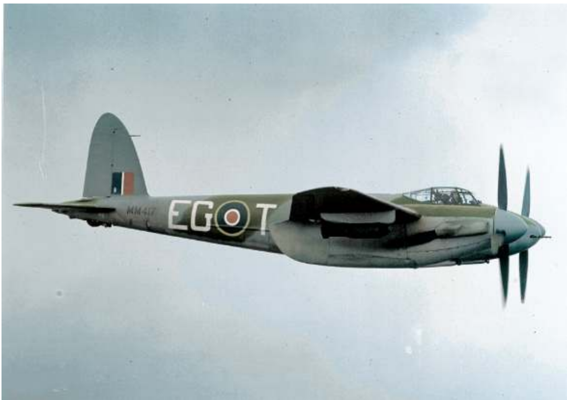
The de Havilland Mosquito employed by the RAF was a brilliant fighter-bomber. Constructed almost exclusively from wood and powered by two Rolls-Royce Merlin engines the aircraft could reach speeds in excess of 400 mph. The type was employed during the low-level raid
