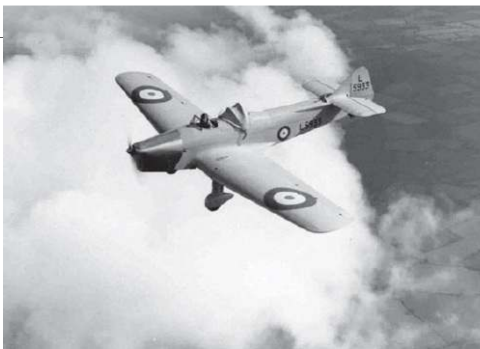
First flying in 1937, the Miles Magister was the RAF's first monoplane designed specifically as a trainer, and with its low wing provided a good introduction to front-line fighters. (RAF Museum, PC98-173-5732-4)
