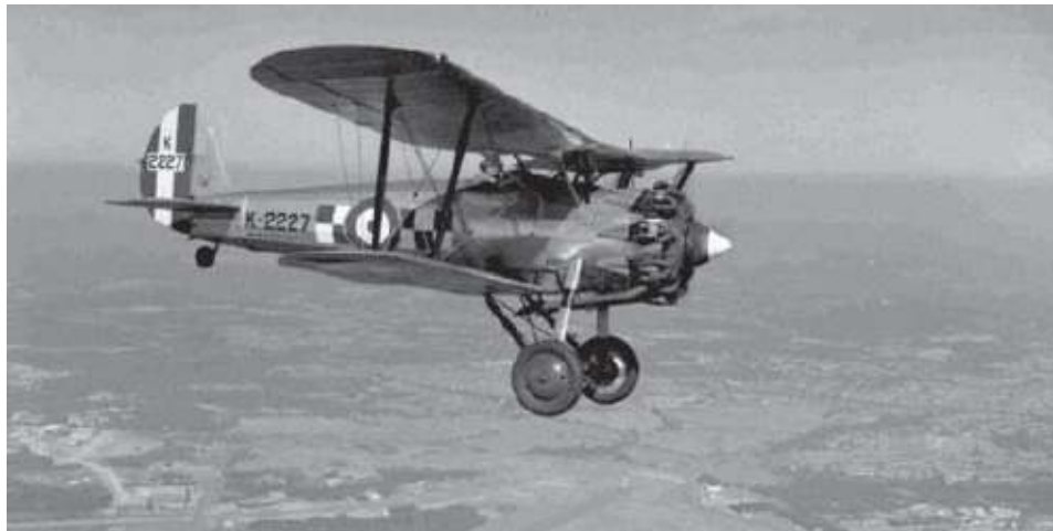
Indicative of the technological standard of aircraft employed by the RAF throughout the inter-war period, the Bristol Bulldog was an open-cockpit, fixed undercarriage, two-gun biplane with a fixed pitch propeller. Still equipping squadrons into the 1930s, the Bulldog was similar in many respects to its Great War predecessors. (RAF Museum, PC71-66-83)
