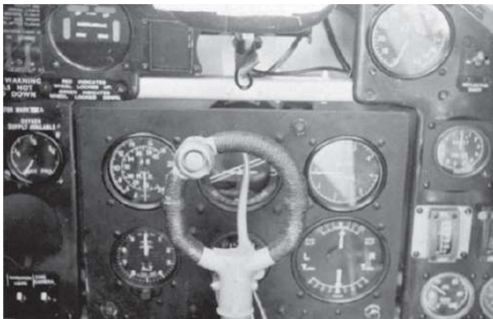
The cockpit of a Hawker Hurricane: the instruments are deliberately set out for the 'selective scan' used in instrument flying, a technique which had developed into an embryonic state in World War I for flying through cloud. The technique involves centring the scan around the artificial horizon, then glancing across at other instruments at regular intervals. (RAF Museum, P010041)
