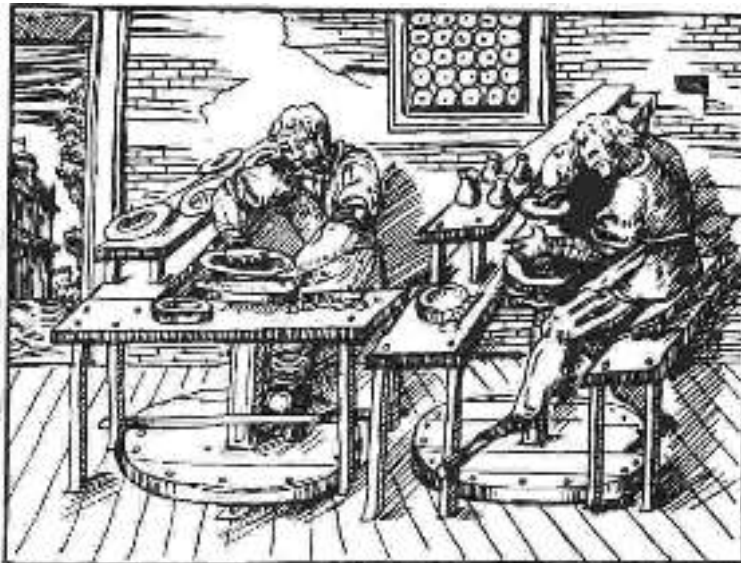
Figure 1.2 Two potters using foot wheels. From an Italian treatise on pottery written by Cipriano Piccolpasso, about 1500 AD. The construction details of the wheel are interesting, it is built from a sort of plywood and can be considered as a forerunner of modern plywood or laminated composite disc flywheels.
