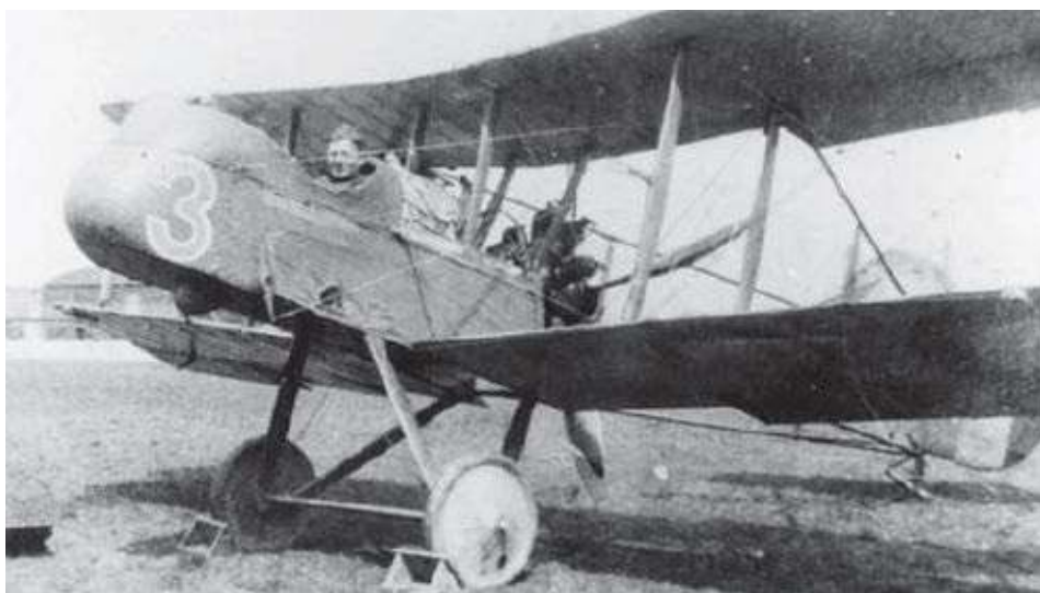
A DH 2 with the engine cowl panels removed, revealing the doped canvas bag that surrounded the fuel tank. (Alex Revell)
