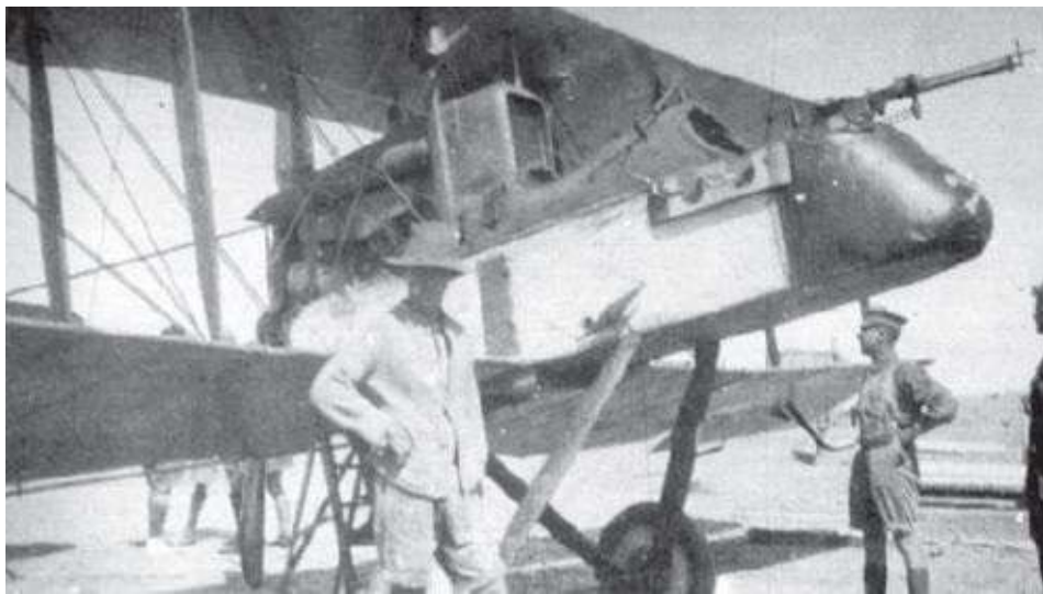
An AMC DH 1A, forerunner of the DH 2, seen here in service with No. 14 Sqn in the Middle East. DH 1As were DH 1s fitted with a 120hp inline Beardmore engine, which generated a top speed of 90mph at sea level. (Aaron Weaver)
