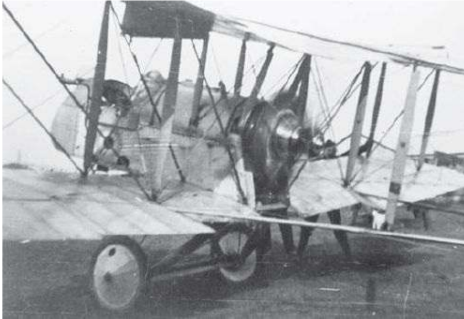
Although slightly blurred, this photograph affords an excellent view of the DH 2 Monosoupape rotary engine spinning with the propeller. At such velocity, the damage wrought by a departing cylinder can be readily imagined. (Colin Owers via Aaron Weaver)
