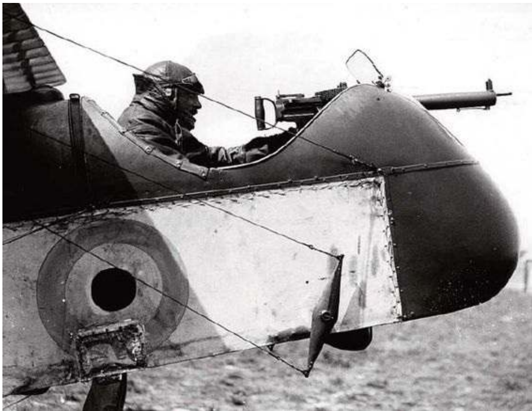
This outstanding close-up photograph of American volunteer pilot Lt Geoffrey H. Bonnell of No. 32 Sqn clearly reveals the DH 2's nacelle and single 0.303in Lewis machine gun. Bonnell would later join the US Army Air Service and command the 147th Aero Squadron. (Aaron Weaver)
